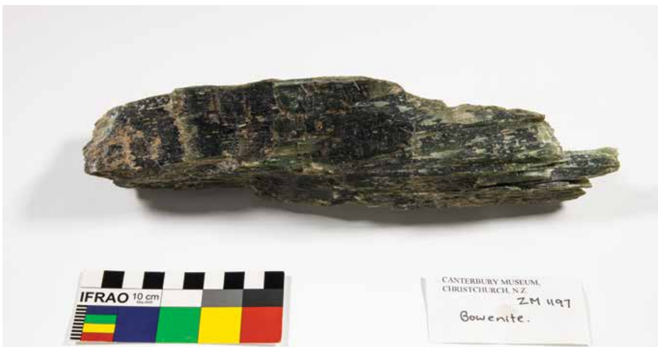
Figure 1. A long piece of unpolished tangiwai that shows its tendency to fracture and flake. Canterbury Museum ZM1197
