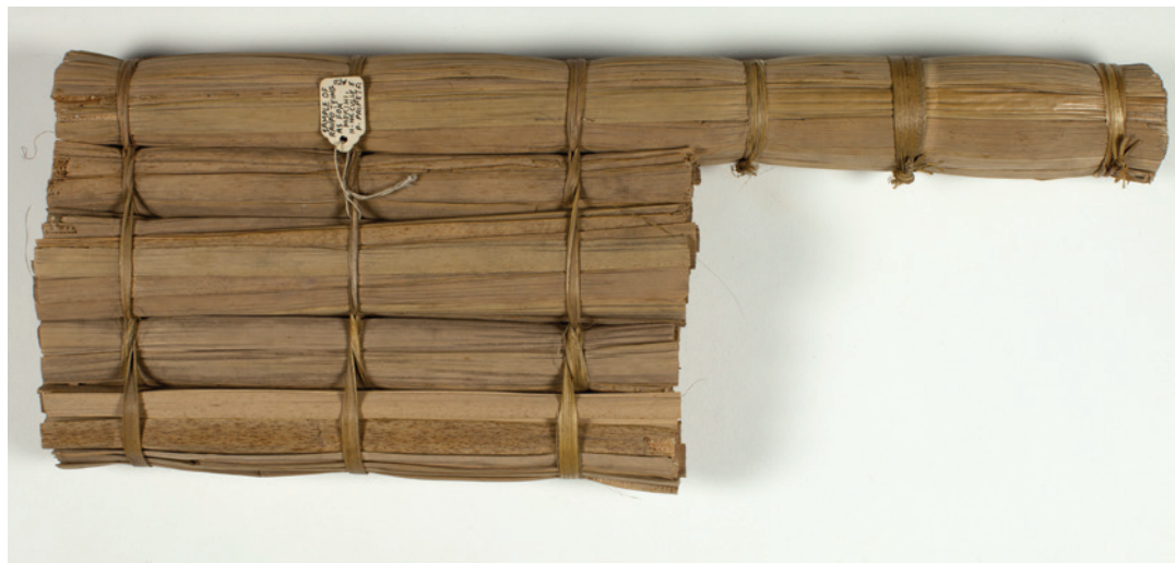
Figure 3. The ‘scientific’ model cross-section to demonstrate how water tightness relied on correctly tied and knotted bundles of raupō. Canterbury Museum E151.210
